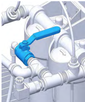
Water valve in closed position
